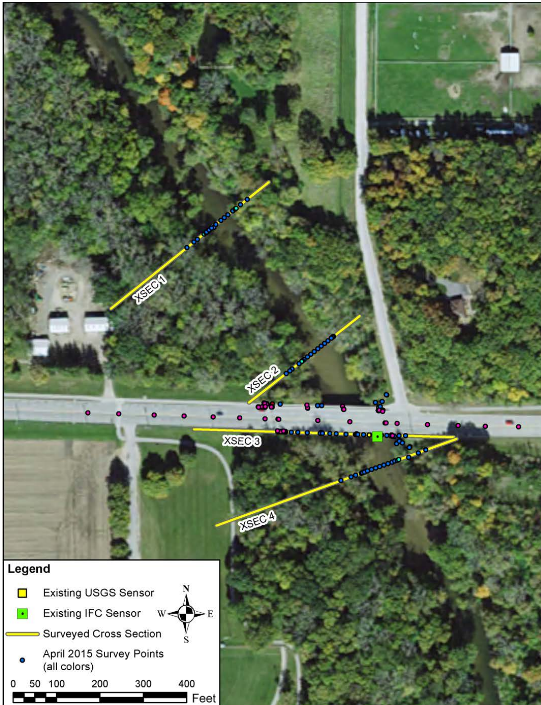
Figure 15: Cross-Section Layout for the South Skunk River at Ames, IA
