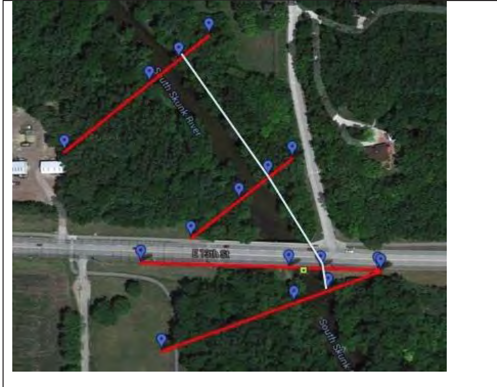
Figure 5. Bankline profiles used for the free-surface slope estimation 2.3 Estimation of Manning's Coefficient
